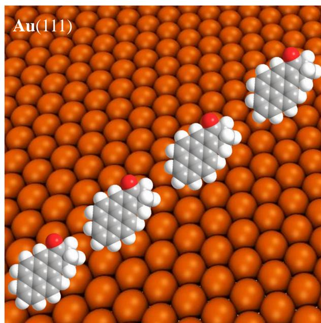
Fig.2 The diagram illustrates self-assembly of polar pyrene to 1D ferroelectric molecular wires driven by dipole-dipole interaction.
