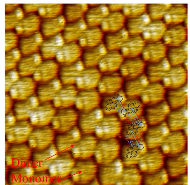
Fig.3 The evolution of 1D wires into 2D ferroelectric ordered array induced by hydrogen bond.
