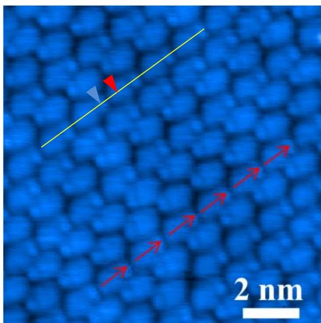
Fig.1 Constant current STM image reveals the molecular arrangement of polar pyrene on Au(111).  $V_{\text{Tip}} = -2.0$  V, 72.6 pA and 77K.
