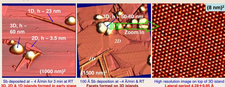
Sb deposited at ~ 4 Å/min for 3 min at RT
