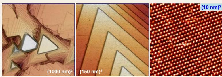
40 nm Sb deposited at ~ 20 Å/min at RT
