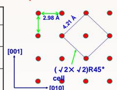
Atomic volume of rhombohedral Sb at normal pressure & RT  $V_0 = 30.21 \text{ \AA}^3$ , whereas in our case, volume of simple cubic structure is  $V = 26.46 \text{ \AA}^3$ . So we have  $V/V_0 = 0.88$
