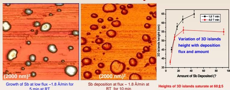
Growth of Sb at low flux ~ 1.8 Å/min for 5 min at RT
