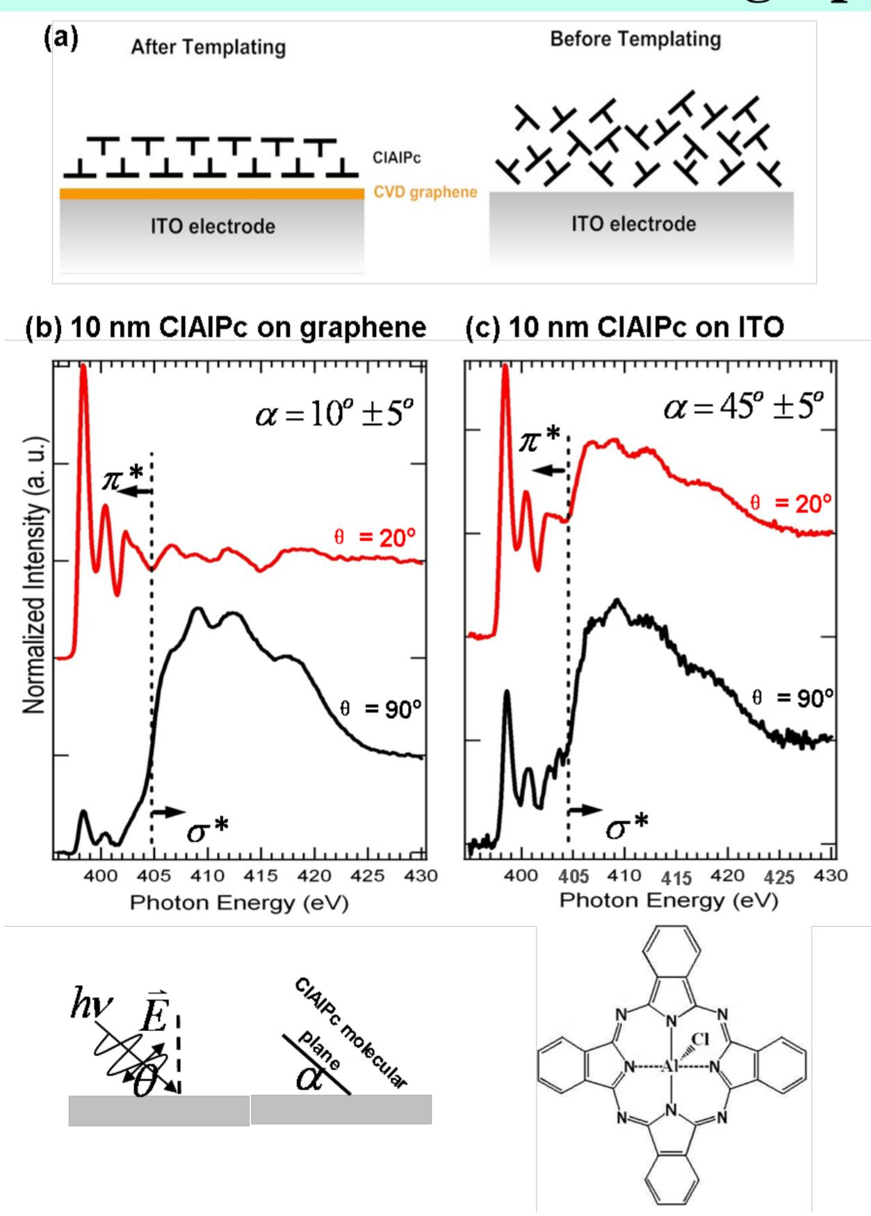
(a) Schematic of the proposed molecular packing structure for ClAlPc molecules before and after templated by CVD graphene. Angular-dependent N K-edge NEXAFS spectra for 10 nm ClAlPc film on (b) CVD graphene modified ITO and (c) bare ITO electrodes. The molecular structure of ClAlPc is shown at the bottom of the Figure.
