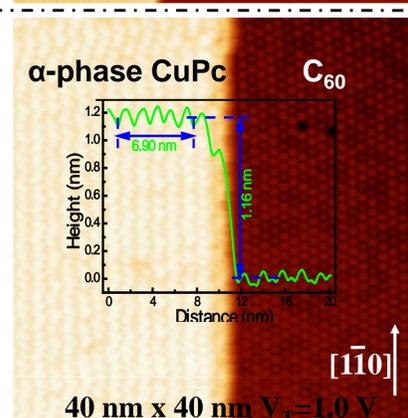
STM image shows poor ordered  $\alpha$ -phase CuPc molecular rows (the left half) along the [1-10] azimuth of hcp C<sub>60</sub> monolayer (the right half). In the molecular rows, CuPc molecules arranged rather disordered. The inserted line profile reveals that the CuPc layer is around 1.16nm high and about 1.4nm wide, indicating that the CuPc molecules are not oriented parallel to the substrate.
