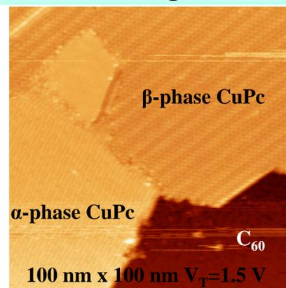
~0.5 ML CuPc on C<sub>60</sub>/Ag(111), two kinds of heterostructures are formed with an angle of 30° relative to each other, labeled as  $\alpha$ -phase and  $\beta$ -phase, respectively.
