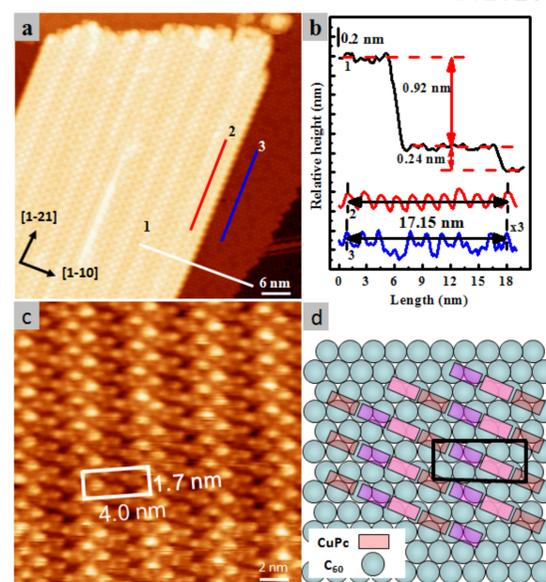
a) STM image of pure  $\beta$ -phase CuPc on C<sub>60</sub>/Ag(111) running along along the[1-21] direction of hcp C<sub>60</sub> ; b) line profiles show  $\beta$ -phase CuPc with a height of 0.92 nm and a width of 1.72 nm; c) corresponding close-up showing the moiré pattern with dimensions of 4 nm and 1.7 nm, the (4 x 1) unit cell containing 3 CuPc and 4 C<sub>60</sub> molecules; revealing a commensurate epitaxy; d) schematic of proposed model.
