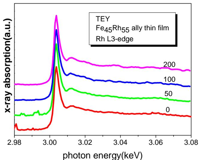
Fig.2 Normalized XAS of a 80 nm thick Fe<sub>45</sub>Rh<sub>55</sub> thin film at Rh L3-edge, collected in sample current mode at a bias of 0, 50, 100 and 200V, respectively.
