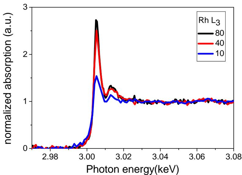
Fig.3 Normalized fluorescent XAS of the 80 nm thick Fe<sub>60</sub>Rh<sub>40</sub> thin film at Rh L3-edge using the proportional counter detector with three different distances from the film.
