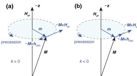
Schematics of the precession of the magnetization M under the total effective field  $H_{eff}$  +  $h_{DMI}$  for (a) k>0 and (b) k<0. All the vectors in the xy-plane are labelled blue. This explains why the dispersion relation is asymmetric.
