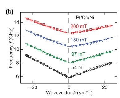
(a) Brillouin spectra recorded at a fixed incident angle of  $\theta$  = 45° (k = 17.3  $\mu m^{-1}$ ) under oppositely oriented external magnetic fields. (b) Asymmetric spin-wave dispersion relation of a Pt(4nm) / Co(1.6nm) / Ni(1.6nm) film showing interfacial DMI at the Pt/Co interface. Dots represent experimental data, while solid lines are theoretical predictions.
