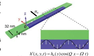
the conservation of energy and momentum, this transition can happen in only one direction, leading to nonreciprocal magnonic transitions. Our finding is useful for stabilizing magnonic circuits.
