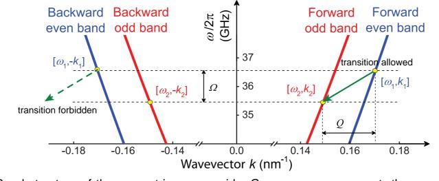
Band structure of the nano-stripe waveguide. Green arrows represent the enrgy and momentum of microwave photons showing possible transitions.
