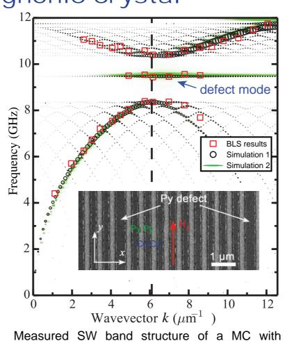
artificial defects. Inset: SEM image of the thin-film-based MC showing defects.
