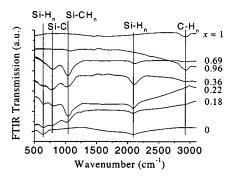
FIG. 1. The FTIR spectra of  $a-Si_{1-x}C_x$ :H at varying carbon fraction x. These are displaced vertically for clarity.
