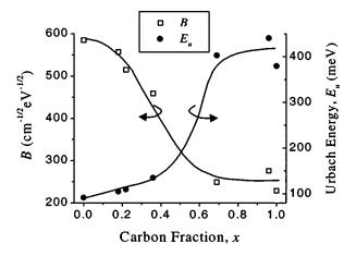
FIG. 5. Variation of the Tauc B parameter and Urbach energy  $E_u$  with carbon fraction x.
