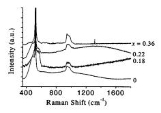
FIG. 2. Raman spectra of Si-rich a-Si<sub>1-x</sub>C<sub>x</sub>:H excited using a visible source (632.8 nm).
