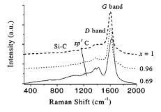
FIG. 3. Raman spectra of C-rich a-Si<sub>1-x</sub>C<sub>x</sub>:H excited using an UV source (244 nm). The line serves as a guide for the eye for the energy shift of the T peak that is assigned to  $sp^3$  C.
