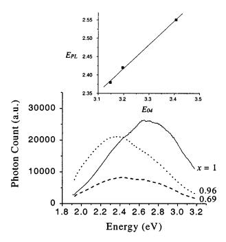
FIG. 6. The room-temperature PL of carbon-rich a-Si<sub>1-x</sub>C<sub>x</sub>:H. Inset: the linear relation observed between the PL peak energy ( $E_{\rm PL}$ ) and the  $E_{04}$  gap.
