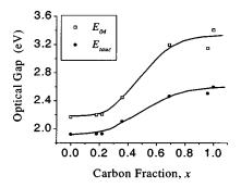
FIG. 4. Variation of the Tauc gap  $E_{\text{tauc}}$  and  $E_{04}$  with carbon fraction x.
