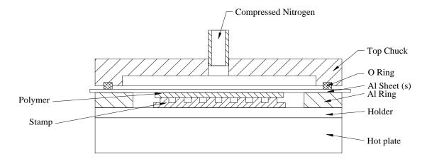
Schematic diagram of this hot embossing system.
