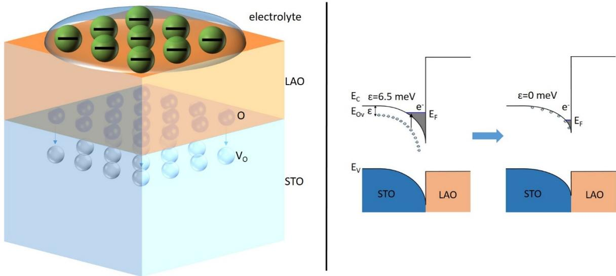
(Left) Figure shows a schematic of the operation of LAO/STO electrolyte field effect device. High electric field drives the oxygen (O) migration into STO to fill some of the vacancies (V<sub>O</sub>). (Right) Change of interfacial energy band structures as a result of electrolyte field effect.
