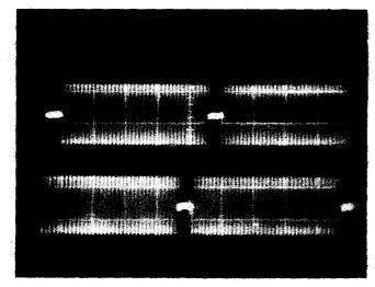
Figure 4. Time delayed pulse modulated 4 kHz sine wave: upper band is original wave (2 V cm<sup>-1</sup>); lower band is delayed wave (5 V cm<sup>-1</sup>); time base is 2.08 ms cm<sup>-1</sup>
