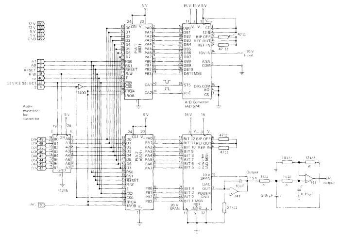
Figure 1. Circuit diagram of analogue I/O board
